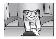
Put the coloured descaling funnel in its place.
